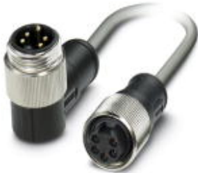
Bus system cable, DeviceNet, 5-position, PUR halogen-free, Gray RAL 7001, Plug angled 7/8"-16UNF, on Socket straight 7/8"-16UNF, Cable length: 0.3 m
